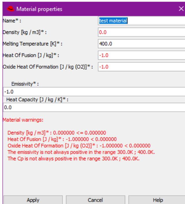
Figure 67 Entry of a user-defined material
