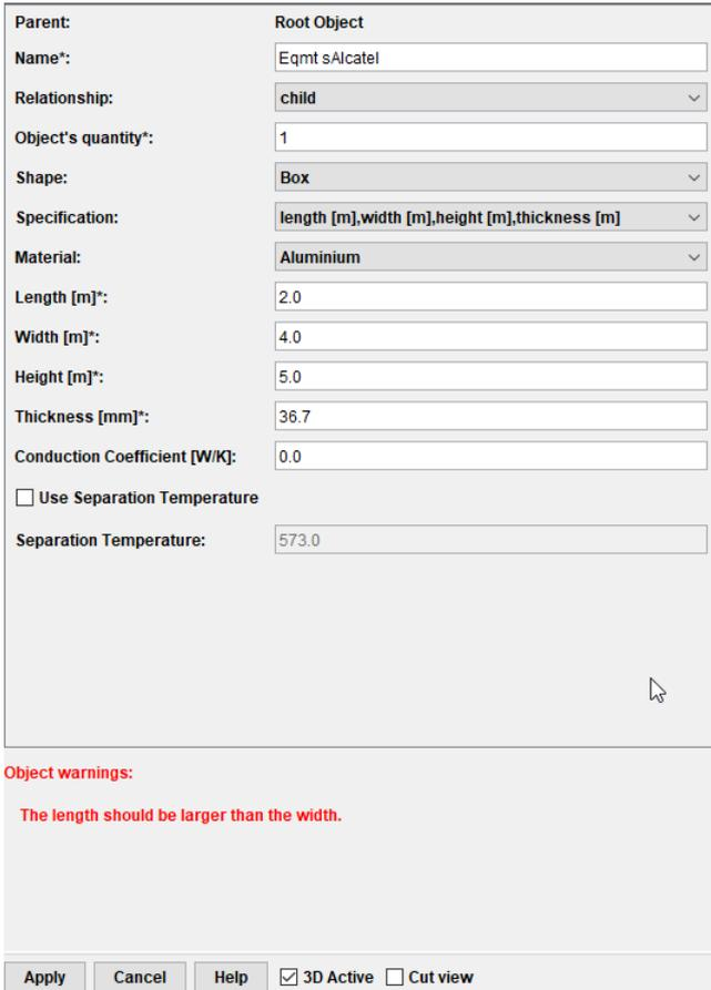
A dialog box for defining object dimensions. It has a "Parent:" field set to "Root Object". The "Name\*" field contains "Eqmt sAlcatel". The "Relationship:" dropdown is set to "child". The "Object's quantity\*" is 1, "Shape:" is "Box", and "Specification:" is "length [m],width [m],height [m],thickness [m]". The "Material:" dropdown is set to "Aluminium".
