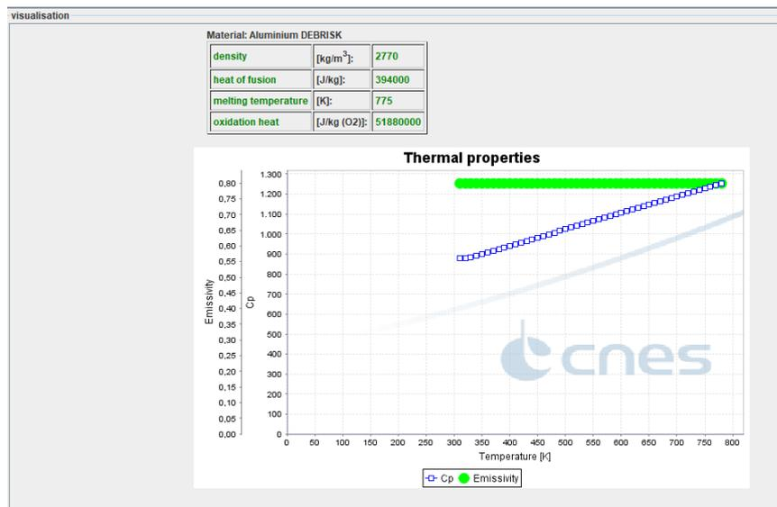
**Figure 38 Materials tab thermal properties graph**
