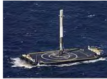
First stage of Falcon 9 Flight 23 landed on autonomous droneship
